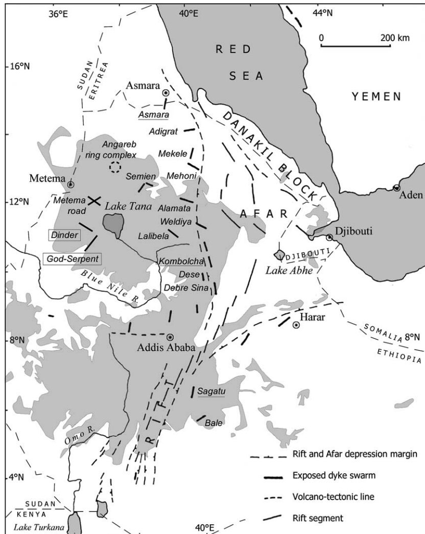
Fig. 1. Location of the main dyke swarms in Ethiopia according to and modified after Mohr and Zanettin (1988). Many dyke swarms reported on this map have not been studied yet, and unreported swarms are likely to exist. Swarm orientations are indicative of the main dyke strikes, although the swarms on the Afar margin display multiple orientations, presumably in response to post-emplacement rotations. Previously studied dyke swarms are underlined (references in the text). The Serpent-God and the Dinder dyke swarms, studied in the present paper, are framed. The Dinder, Metema, Lalibela and Mekele swarms were not included in Mohr and Zanettin's survey. The current exposure of the Trap Series is from various sources.
