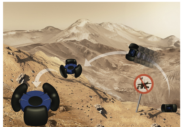
Fig. 3. Artist's view of a hopper in a Valles Marineris-type landscape (no vertical exaggeration). The maximum jumping height on Mars with the currently considered mechanisms is anticipated to be 4 m.
