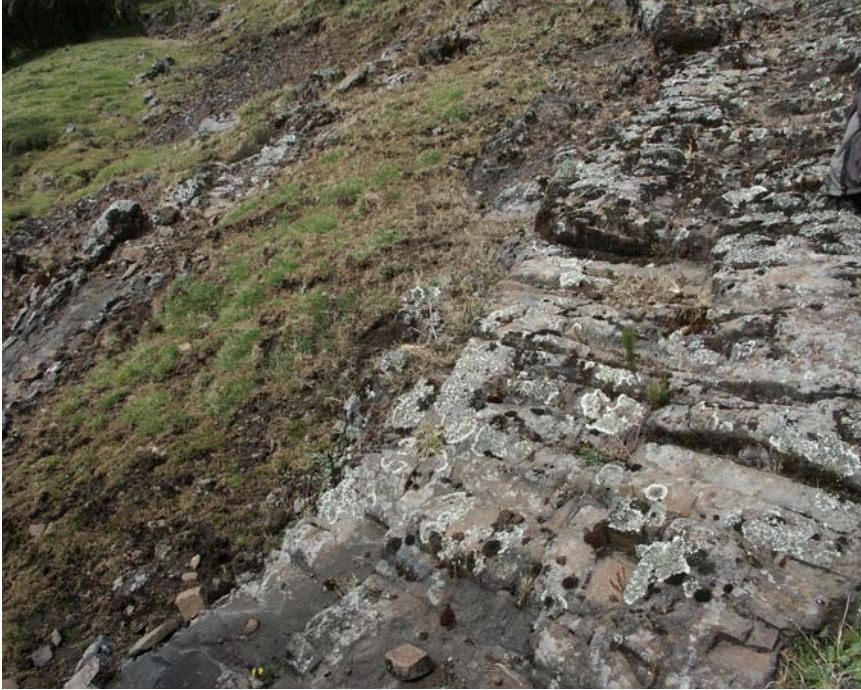
Figure 4.9b Field photograph of columnar jointing due to cooling effect on Basaltic dyke; strike N5°E, thickness 1.8 m. Water comes out at the contact of dyke and country rock
