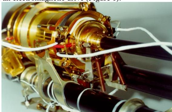
Fig.1. MUPUS - electromagnetically driven insertion device.
