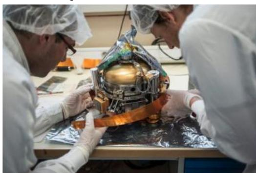
Figure 1: Integration of the SEIS sensor heads. The sphere includes the 3 long period seismic sensors, while the 3 short period are located on 3 boxes around the leveling ring
