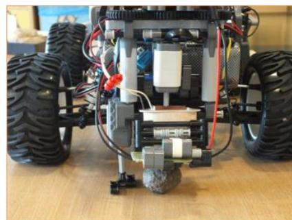
Fig. 3. The Husar-5 rover when coil of the magnetic experiment is in lowered position, under it the siderite-candidat
